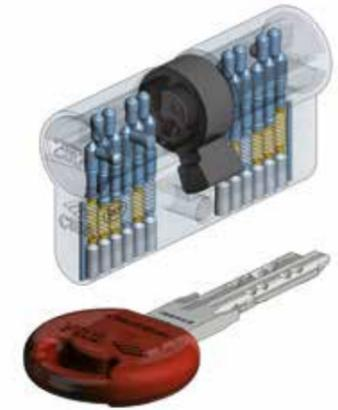
The built in clutch function as standard, allows the cylinder to be operated even if a key is inserted in the opposite side of the cylinder.
